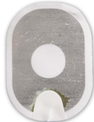
Figure 3: Gel almost completely separated from backing.
