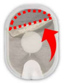
Areas of missing gel
